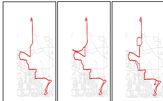
Flexible routing allows transit services to divert from a fixed route to pick up and drop off passengers closer to their origin and destination points. TARTA’s Call-a-Ride services in Perrysburg, Maumee and Sylvania, and the Bedford Dial-a-Ride are examples of flexible route service.
