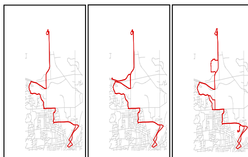
Flexible routing allows transit services to divert from a fixed route to pick up and drop off passengers closer to their origin and destination points. TARTA's Call-a-Ride services in Perrysburg, Maumee and Sylvania, and the Bedford Dial-a-Ride are examples of flexible route service.
